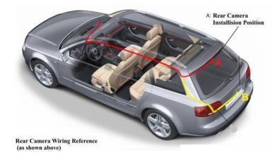
Red Wire: This wire provides 12 Volt (V) power to your rear camera. This can be connected to any 12V power source on your vehicle. However, it's recommended to connect to your reverse lights so the rear camera only turns on when the vehicle is in reverse.
